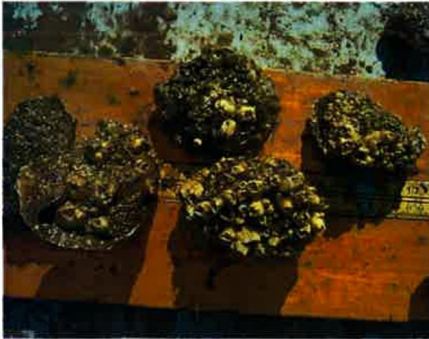
Example of fouling problems
