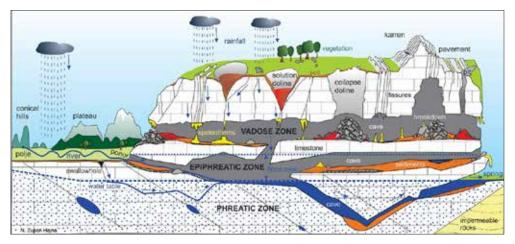
Figure 2.1.2: Conceptual model of the water flow in a karst aquifer with the main surface and underground geomorphological features (from N. Zupan Hajna, 2021)
